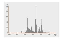
DULUX S 7 W/830 | DULUX S 9 W/830 | DULUX S 11 W/830
